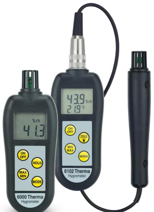
**INSTRUMENT OPERATION** - The instrument is switched on by pressing the ON/OFF button. To obtain accurate humidity measurements, allow the instrument to stabilise in the environment for a minimum of one minute. To maximise accuracy, allow airflow across the sensor.
